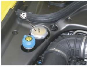
. Unscrew the cap (C) on the oil tank and remove.
