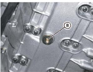
. Unscrew the cap (B) on the crankcase sump and drain all the oil.
