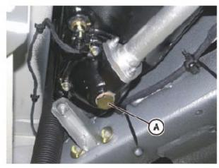
. Unscrew the oil draining cap (A) on the tank.
