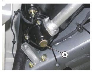
· Screw the lower cap (A) onto the engine oil tank.
