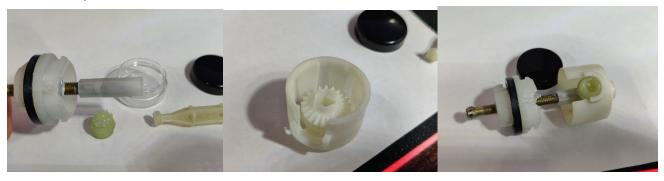
**Step 10:** Now simply slide the "Stack" of parts together with the drive gear aligned to the curved slot in the knob. Everything should "snap" together easily. Turn You can insert the driveshaft into the drive gear and turn by hand to verify function.
