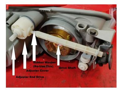
Use a small pick to remove the Adjuster Cover by gently prying the sides up to unlatch from the old Adjuster Knob. (See below)
