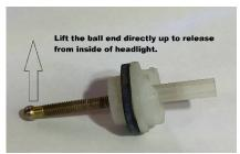
**Step 4:** Remove the old Knob (if its still somewhat solid) by turning counterclockwise. This will only turn around 45\*. Then pull back to remove from housing. The Adjustment rod will now need to be disengaged. Do this by lifting the "ball" end of the rod up.
