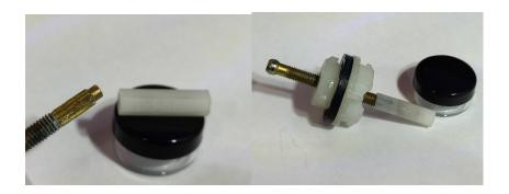
**Step 9:** Almost done. Now coat the original drive gear and the drive shaft end with grease. Also coat the internal gear on both sides. You can then use grease to hold the Cover, Internal Gear, and drive gear together for assembly.
